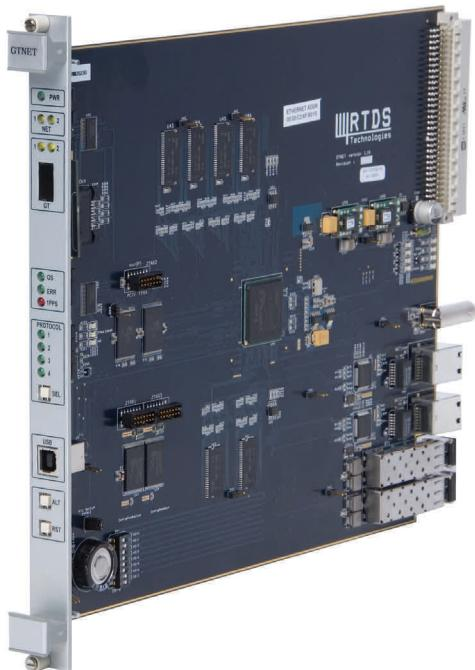
The GTNET card occupies a single slot of an RTDS Simulator rack and draws power from the backplane. The card transmits and receives signals from a PB5 processor through one of the GT ports on the rear of the processor card. Other GT-I/O cards can be connected in daisy chain to the GTNET and serviced through the same PB5 GT port.
